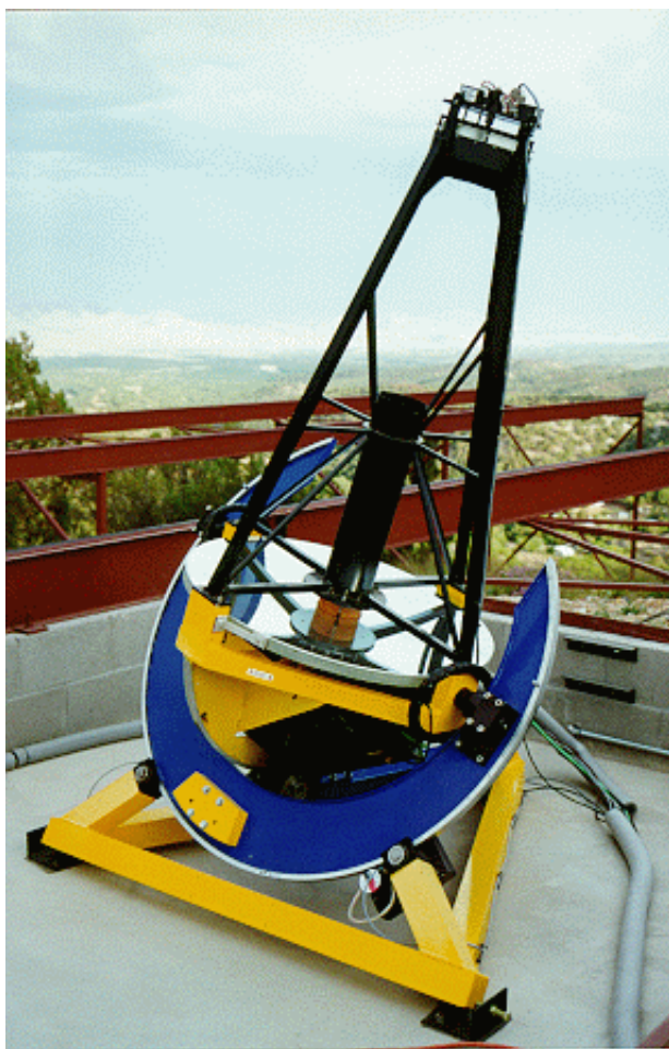
FIG. 2.—The 0.80 m APT at Fairborn Observatory. This telescope, along with a similar 0.75 m APT, is dedicated to a long-term program of monitoring luminosity cycles in Sun-like stars. The black box mounted behind the primary mirror is the automated photometer.
