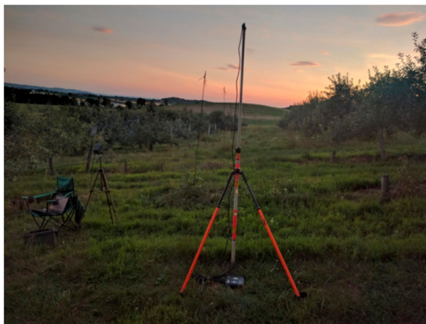
Figure A1. The Pettersson D500x (center) with microphone raised 2.4 m high on a tripod. The AR125 (left) mounted on a lower tripod. Location is at the organic orchard with tree line.
