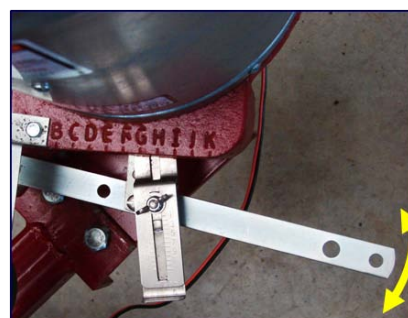
Fig. 2. Left Photo: Area between Herd® spreader hopper and four-bladed fan where stainless steel agitator wire connects to the screw above the fan blades. Right Photo: Close-up image of agitator wire properly positioned with the screw in the middle of the wire hook.
