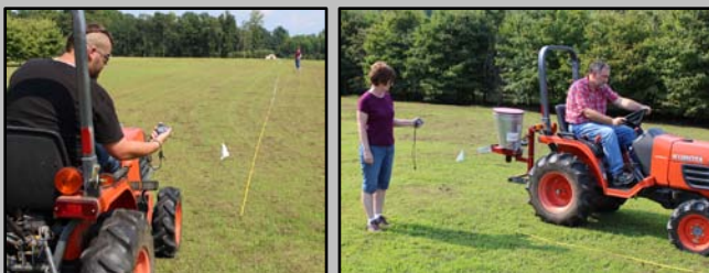
Fig. 2. Travel time can be timed by the vehicle operator ( left photo ) or with the help of another person ( right photo ).
