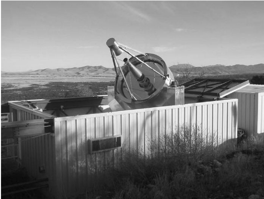
FIG. 1.—TSU 2 m AST at Fairborn Observatory. The telescope is housed in a barn-like enclosure with a top section that rolls off to the north. The echelle spectrograph is in an insulated shipping container to the south.
