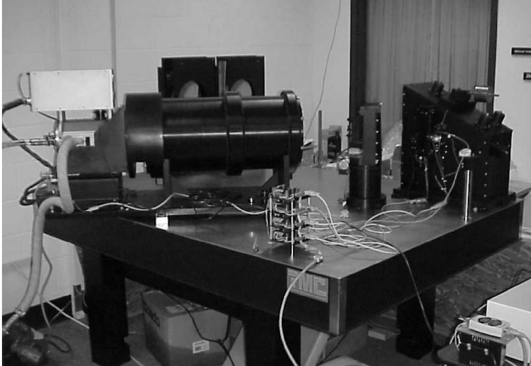
FIG. 2.—Echelle spectrograph for the TSU 2 m automatic telescope assembled in the lab at TSU.
