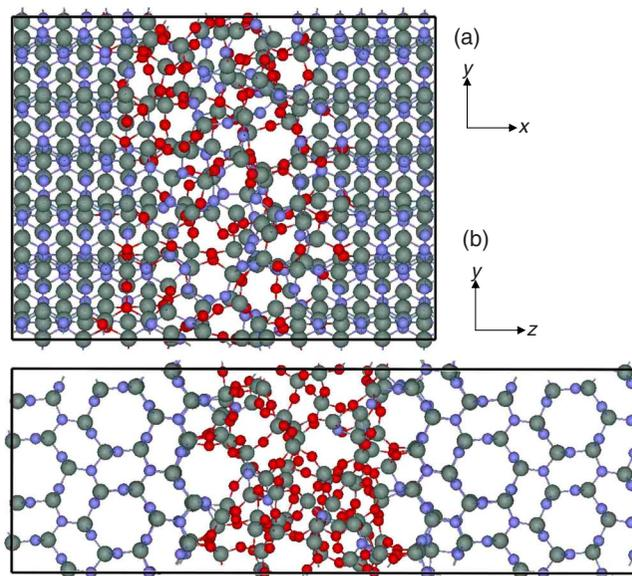
FIG. 1. (Color online) Comparison of the two IGF models in  $\beta$ -Si<sub>3</sub>N<sub>4</sub>: (a) the 798 atom basal model and (b) the 907-atom prismatic model.
