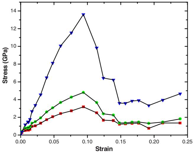
FIG. 2. (Color online) Stress vs strain of the prismatic model under uniaxial extension in the  $z$ -direction. Each data point is collected after full *ab initio* relaxation using VASP at a given strain. The  $xx$  and  $yy$  components of the strain are also shown.
