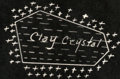
Fig.1 Diagrammatic representation of colloidal clay crystal with its lamellar nucleus or micelle, its innumerable negative charges, and its swarm of exchangeable cation. Under the influence of an electric current such a particle will move toward the positive electrode.
