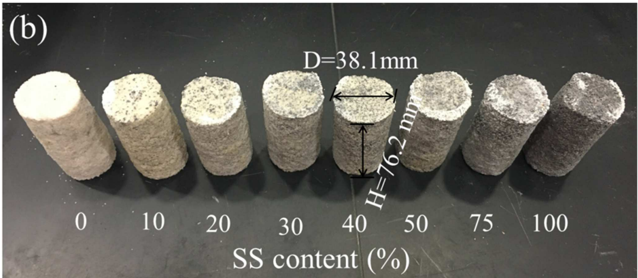
Fig. 1 Materials used in this study: (a) raw SS, (b) MICP-treated SS-sand samples
