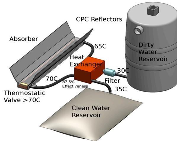
**Figure 1.** Labeled schematic of the primary components of a flow-through solar water pasteurizer.
